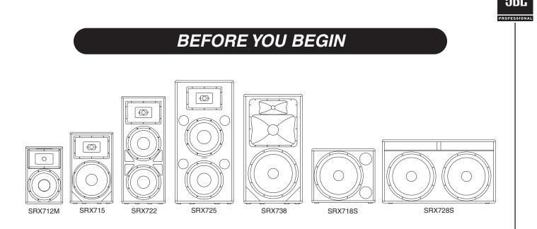
The SRX700 speakers covered by this manual are not intended for fixed installation in outdoor or high moisture environments. Moisture can damage the speaker cone and surround and cause corrosion of electrical contacts and metal parts. Avoid exposing the speakers to direct moisture. Keep speakers out of extended or intense direct sunlight. The driver suspension will prematurely dry out and finished surfaces may be degraded by long-term exposure to intense ultra-violet (UV) light.
