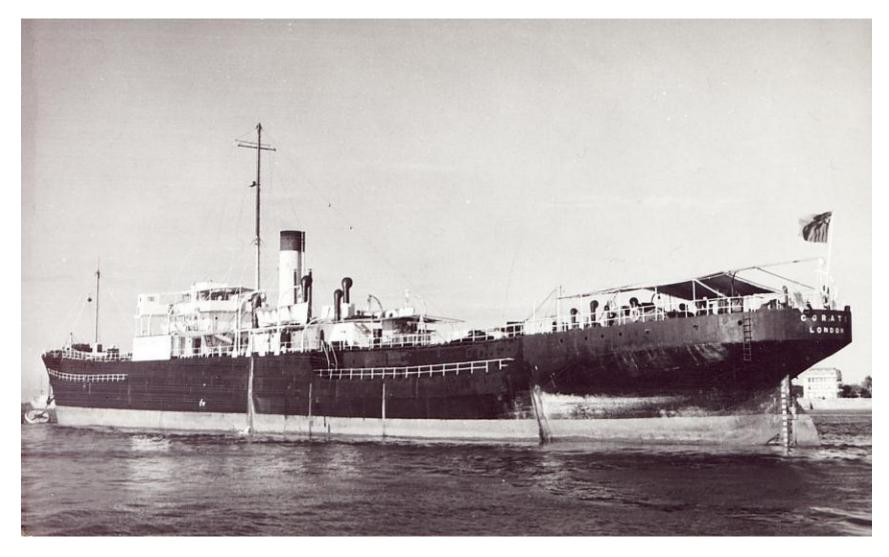
Completed 11/1918,5563grt, by Sir James Laing & Sons, Sunderland (672) as WAR JEMADAR for the Shipping Controller, U.K. (Hunting & Sons), London,GBR 'Z' type tanker, placed in service as a fleet oiler under naval direction
