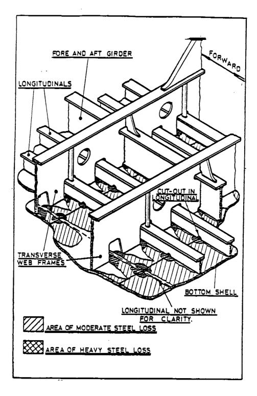
Figure 22: TYPICAL BOTTOM SHELL LOSS PATTERNS
