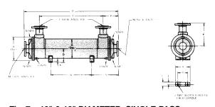
Fig. 7  $\,$  10" & 12" DIAMETER, SINGLE-PASS
