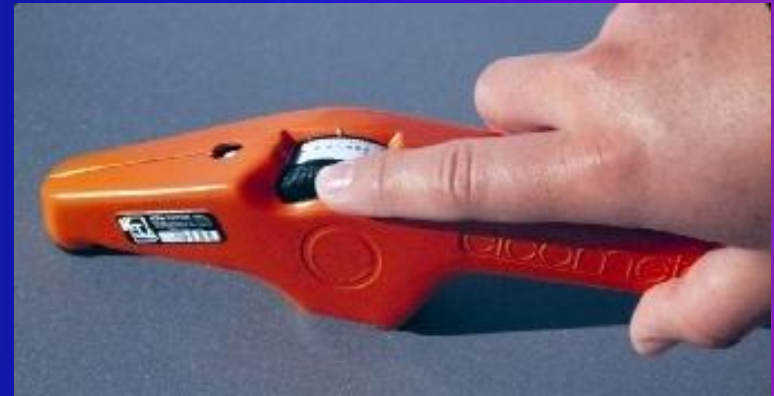
Measuring Base Metal Effect with Type 1 DFT Gage
