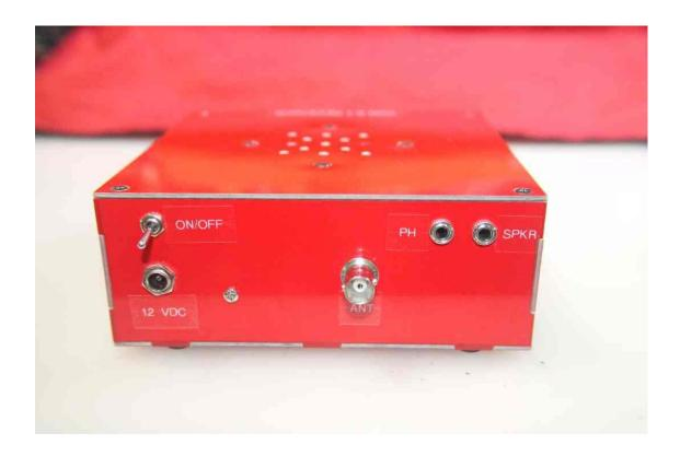
About then, our fantastic kit designers came up with the AAOZZ PC material enclosures and I obtained one of each size that was available at the time. The PC board for the SSB 6.1 was a bit too large for the small (Little Blue Box) enclosure, so I did a quick layout to see if it would go into the medium (Little Red Box) enclosure and fortunately there was enough room to put everything in there.
