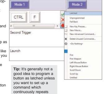
**Fall back:** By default, any commands that you program to a button in the basic mode or shift state will automatically be carried over to the other modes or shift states. When Fall back is ticked, this is the case. You will probably want to assign different commands to individual buttons in different modes.
