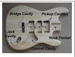
Figure 2.1 Body Cavity Locations
