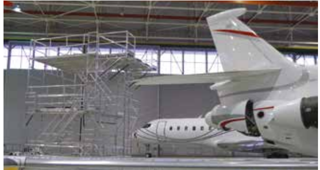
Shanghai Hawker Pacific recently completed construction of a new tail dock which allows it to perform maintenance on critical areas of Falcon aircraft.
