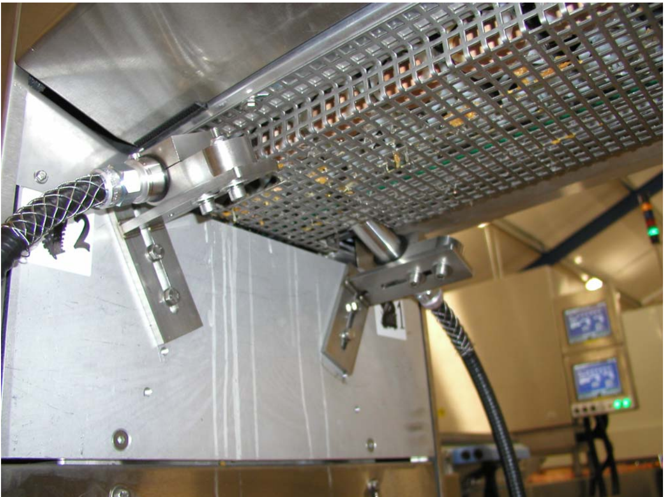
Figure 23. Printheads brackets for the Ardentia 2 track.
