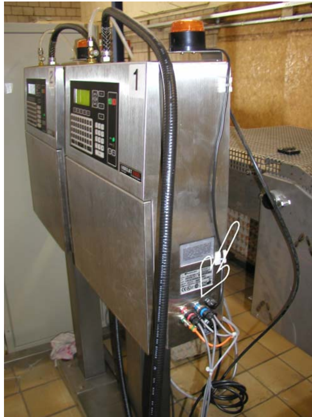
Figure 7. Place of encoder connector at the Excel printer.
