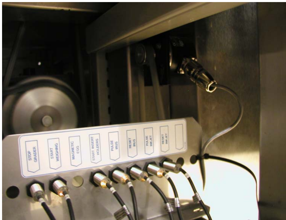
Figure 13. Synch-flag and product detect on an Ardentia / Selecta
