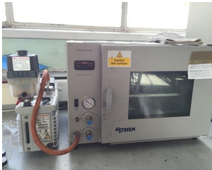
(c) Vacuum treatment to remove bubbles
