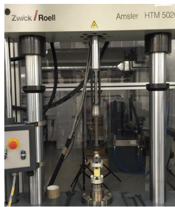
Figure 5.7 Test configurations of high strain rate tensile tests of fabric strips
