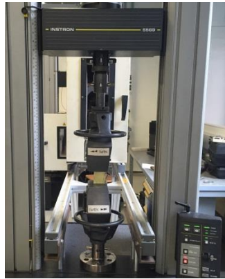
Figure 5.4 Fabric tensile tests configuration
