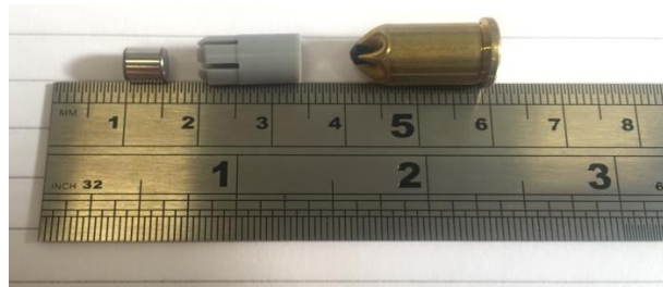
Figure 6.2 (a) steel projectile (b) plastic sabot (c) cartridge
