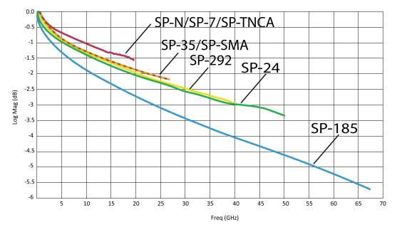
Maury StabilityPlus™ 36" Cable Assembly Typical Insertion Loss
