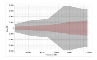
S11\_mag measured on a  $50\Omega$  termination SP-35-MM-36 shown in red; leading global competitor shown in grey
