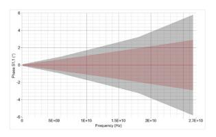
S11\_phase measured on a short circuit termination SP-35-MM-36 shown in red; leading global competitor shown in grey
