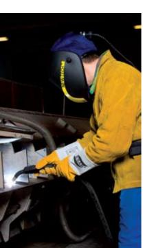
Traditionally, the most popular processes for the welding of stainless steels have been manual arc followed by MIG, TIG and submerged arc. Solid wire is faster than manual arc, but can lack appeal due to spatter levels, a heavily oxidised weld deposit or fusion defects related to low current positional welding using dip transfer.
