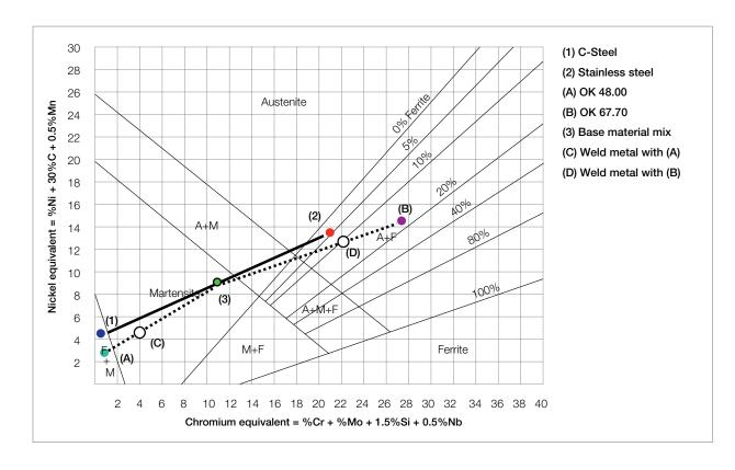
structure with some ferrite. As discussed in the "Ferrite in weld metals" section this will produce a very crack resistant and ductile weld. Typically overalloyed consumables of the (in wt.%) 23Cr 12Ni (with or without Mo) and 29Cr 9Ni types are used. A duplex filler can in most cases also be used with good result.
