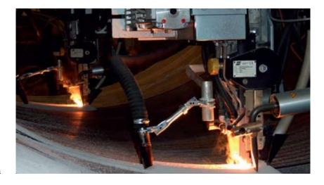
melts the surface of the base material and the strip electrode end, which is dipping in the slag and the flux. The penetration is less for ESW than for SAW since there is no arc between the strip electrode and the parent material.
