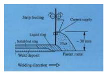
Figure 1.Principles of electroslag strip cladding.
