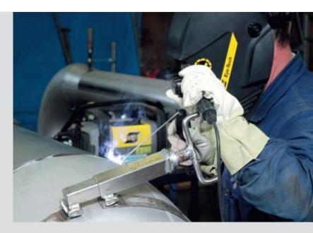
OK 61.20 used for the vertical down welding of water supply piping in the pipeshop at a paper and pulp plant (AISI 304, 2.5 mm wall thickness). The remote control on the CaddyArc portable inverter is used to prevent burn-through by controlling the arc which is directed at the root of the joint. Welding is carried out in the two o'clock position while the pipe is rotated upwards, manually.
