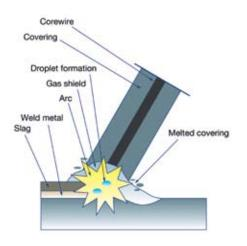
Principle of manual metal arc werlding.
