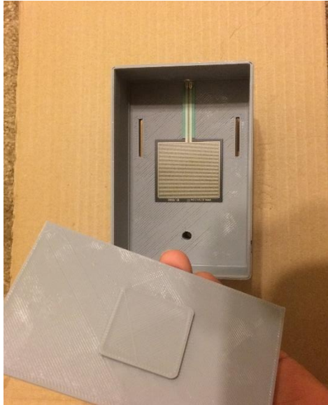
Figure 7: Pressure sensor used as a weight sensor
