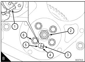
**Caution:** The fuel pump gear must be fitted to the engine before the crankshaft is rotated.
