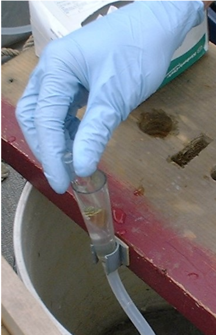
Figure 3. Using a sampling cone to fill a vacuum vial for spectrophotometric analysis.
