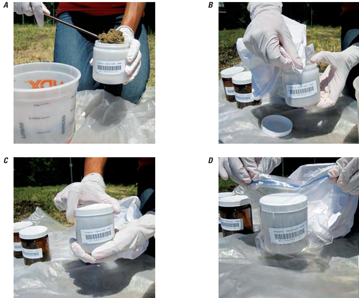
Figure 12. Steps for collecting samples for inorganics screening analysis (sample container 02).
