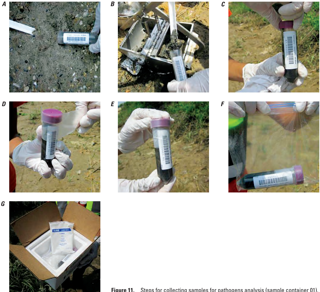
Figure 11. Steps for collecting samples for pathogens analysis (sample container 01).
