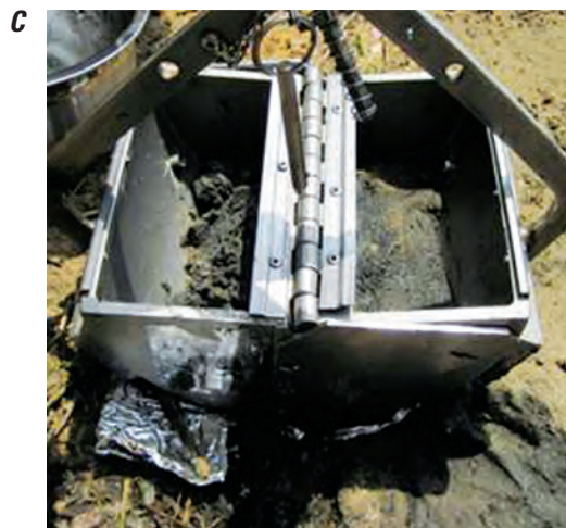
Figure 10. Steps for collecting bed sediment samples using a Petite Ponar sampler.
