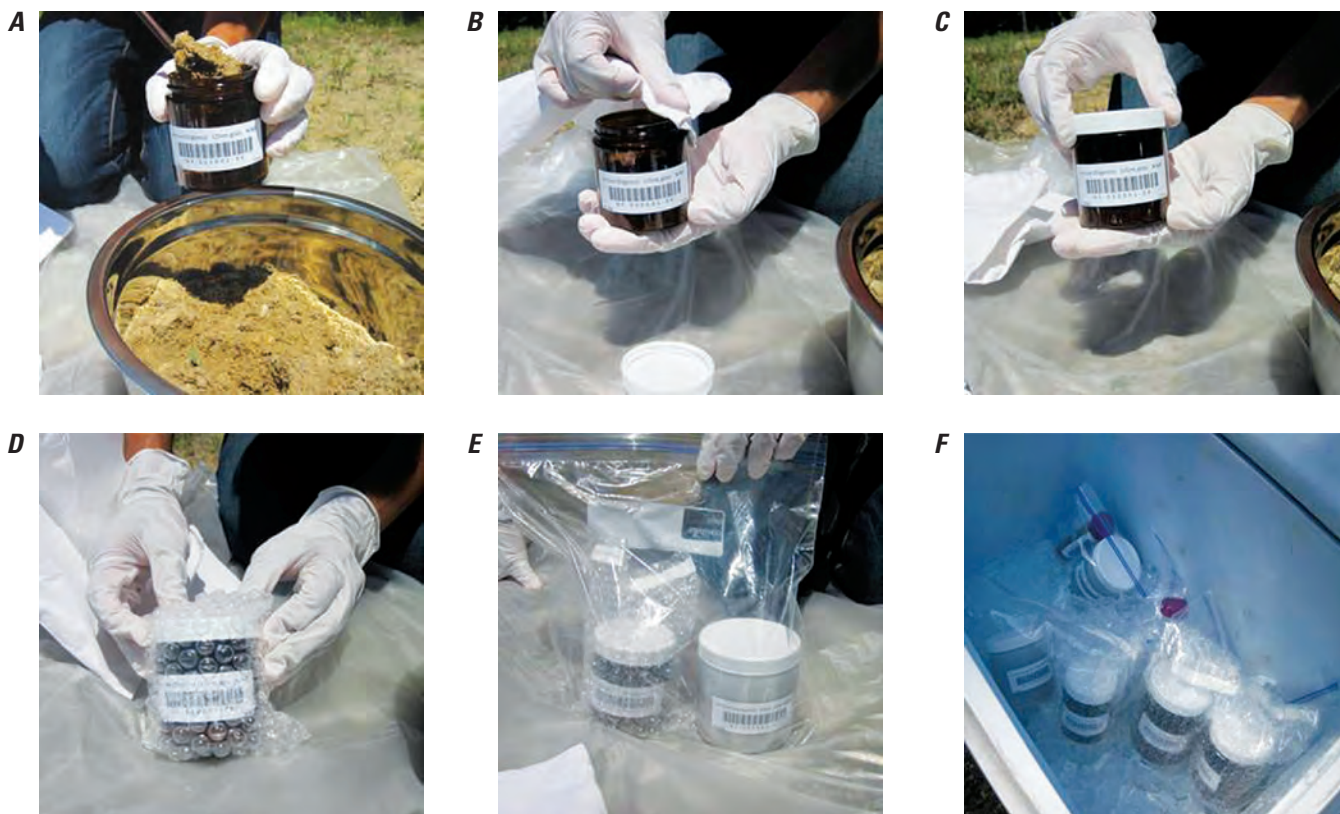
Figure 17. Steps for collecting samples for organics chemistry archive (sample container 08).
