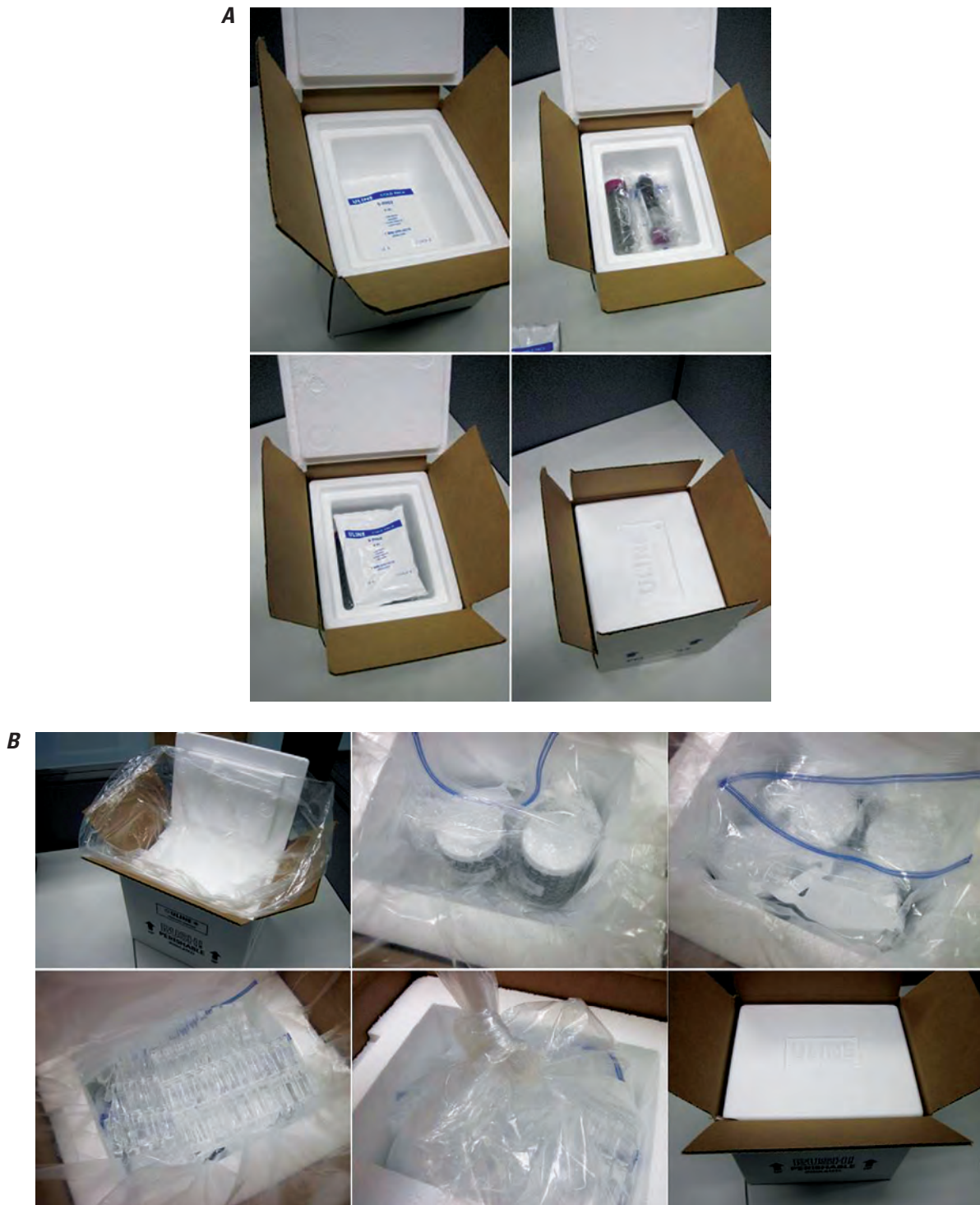
Figure 19. Examples of foam shipping coolers packed to efficiently utilize space and minimize breakage for A , pathogen samples, and B , organic geochemistry samples (use the same method for inorganic geochemistry samples [not shown]).
