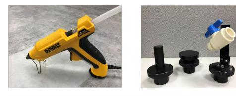
Isopropyl alcohol acts as a quick release agent to remove the glue from samples.
