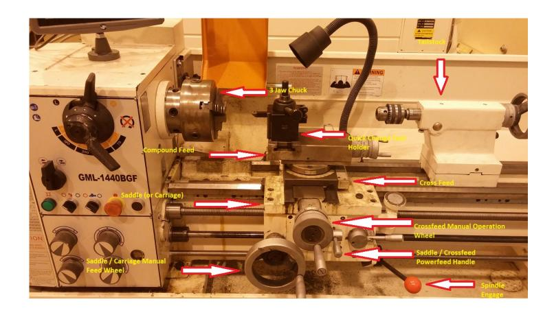
3-Jaw Chuck: Used to hold work (material) to be machined.
