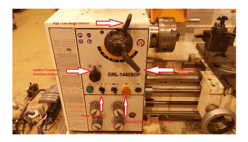
**<u>High / Low Range Selector:</u>** Use to change High / Low range of Spindle Speed Selector.
