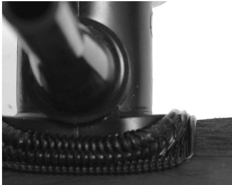
FIG. X2.12 Saddle Fusion Joint
