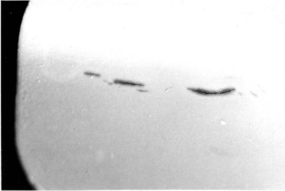
FIG. 7 Example of Type II, Class C, Indication
