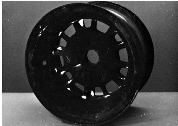
FIG. 4 Example of Type I, Class D, Indication
