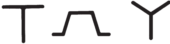
FIG. 1 Typical Cross Sections of Line Post Types
