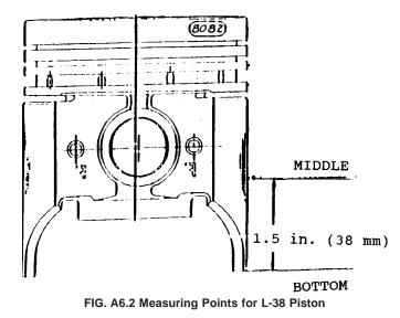
A6.6 Calculate the sleeve bore diameter to be used for the piston-to-sleeve clearance using the middle and bottom transverse measurements according to Table A6.1.
