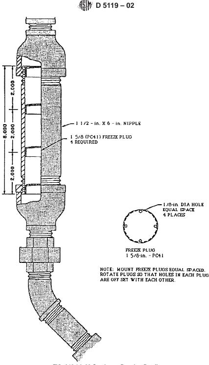
FIG. A10.1 L-38 Crankcase Breather Detail
