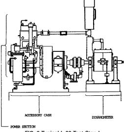
FIG. 2 Typical L-38 Test Stand
