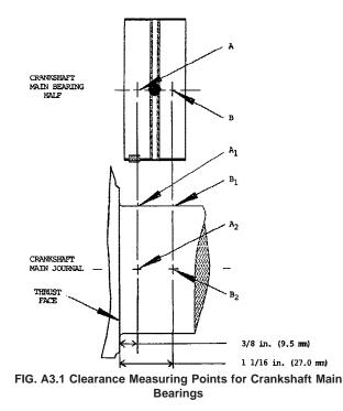
A3.5 Mount the crankshaft on a workbench with the axis horizontal and with the connecting rod bearing journal vertically upward, simulating the TDC position in the engine.
