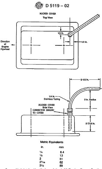
FIG. 4 Rocker Cover Air Inlet for Ventilation of the L-38 Engine Power Section Crankcase
