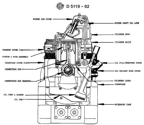
FIG. 1 Sectional View of L-38 Engine Power Section
