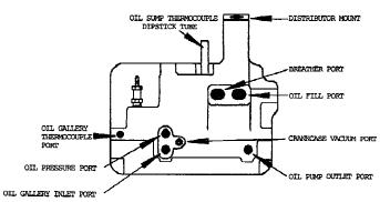
FIG. 6 Oil Gallery Side Cover for the L-38 Engine Power Section
