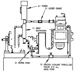
FIG. 9 Cooling System for L-38 Engine Power Section
