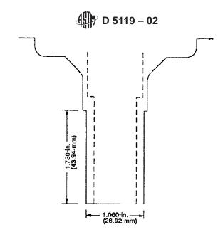
MODIFY TO SPECIFICATION SHOWN FIG. A12.2 Modified Ford Distributor Housing
