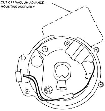
FIG. A12.1 Modified Ford Distributor Housing
