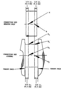
FIG. A2.1 Clearance Measuring Points for Connecting Rod Bearings
