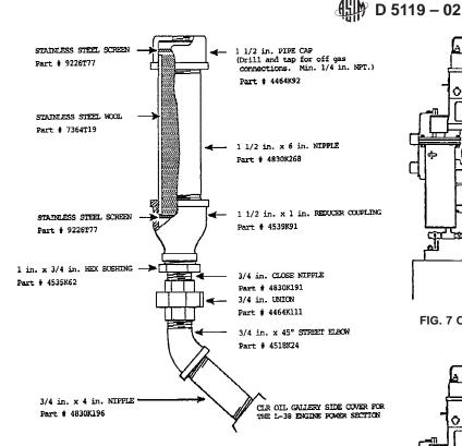
Note 1—See footnote 19 for a source of the parts numbered as shown. FIG. 5 L-38 Crankcase Breather Detail
