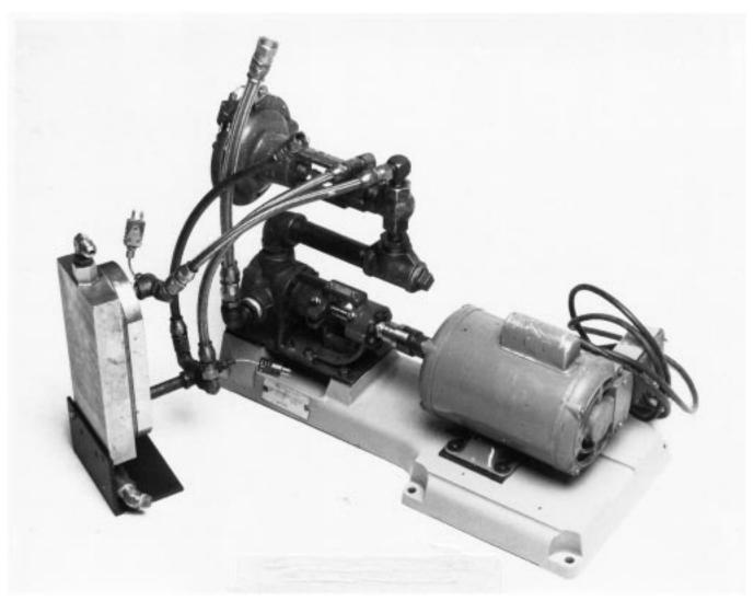
FIG. 5 Sequence IIIE Test Engine External Oil-Cooling System
