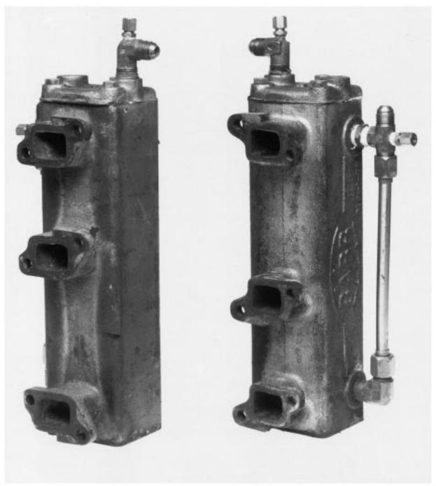
FIG. 12 Sequence IIIE Test Engine Water-Cooled Exhaust Manifolds
