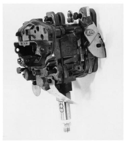
FIG. 3 Sequence IIIE Test Engine Carburetor
