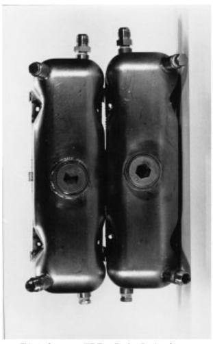
FIG. 17 Sequence IIIE Test Engine Rocker Covers
