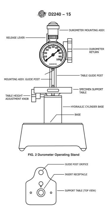
TYPICAL TABLE INSERTS USED FOR POSITIONING TUBING, O-RINGS AND SMALL SPECIMENS
