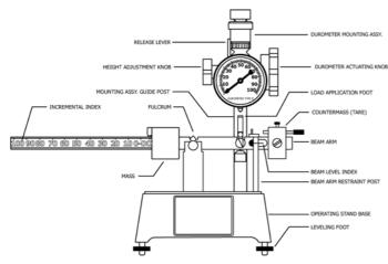
FIG. 5 Example of Durometer Calibration Apparatus
