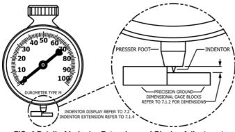
FIG. 4 Detail of Indentor Extension and Display Adjustment
