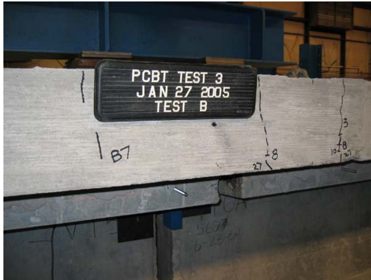
Figure 23. Initial Cracking in Deck, Test 3
