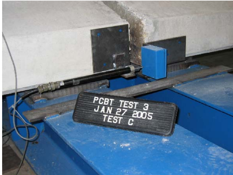
Figure 8. LVDT Used in Static and Cyclic Tests
