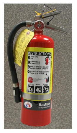
Provide a fire extinguisher, rated at least 2A:10B:C, and be sure to install it correctly. Your fire extinguisher needs to be serviced annually, and after discharge, by a licensed technician and must have a State Fire Marshal Service Tag.
