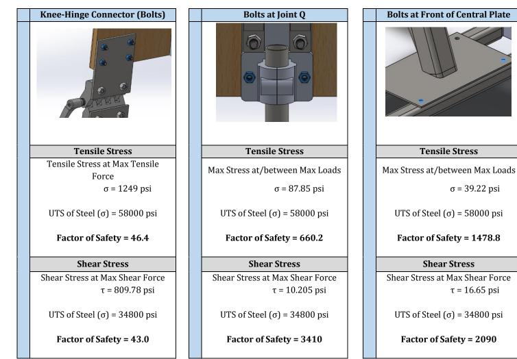
Figure 37: Results of stress analysis of critical components of the design.
