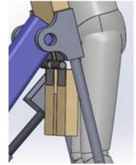
Figure 14: Thigh board adjusted at a position enabling the user to flex the knees.
