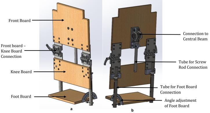
Figure 28: (a) Front and (b) rear views of front board.
