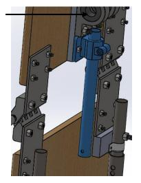
Figure 29: Tube connecting the screw rod to the front board.
