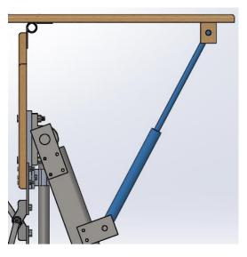
Figure 35: Side-view of tray connector.
