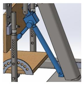
Figure 33: Screw Rod Mechanism.
