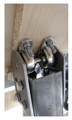
**Figure 41: Center Beam Pivoting Connection.**
