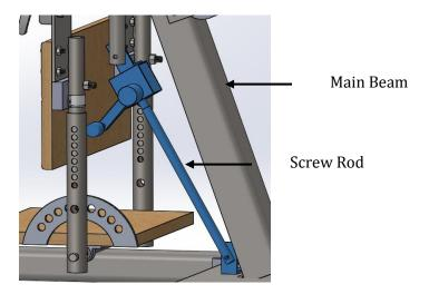
Figure 24: The screw rod is now placed in the middle of the device.
