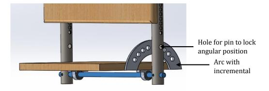
Figure 32: Mechanism used to adjust and lock footboard at different angles.
