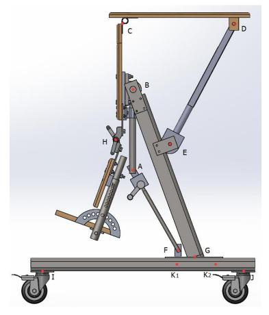
Figure 36: Joints (Letters on Diagram) whose forces were identified after statics analysis.
