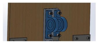
Figure 30: Bearings are used to connect to a pin on the central beam to allow the Front Board to pivot.
