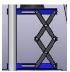
Figure 18: Scissor Jack used in Design 2 to provide growth adjustability.
