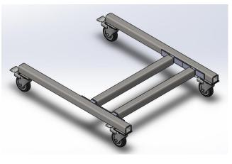
Figure 26: Base frame made of square tubing.
