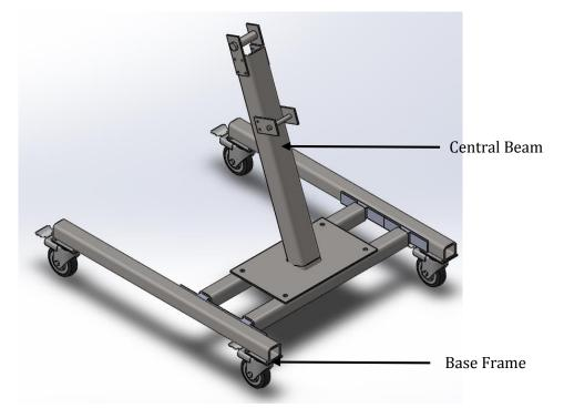
Figure 25: Isometric view of Frame Assembly.
