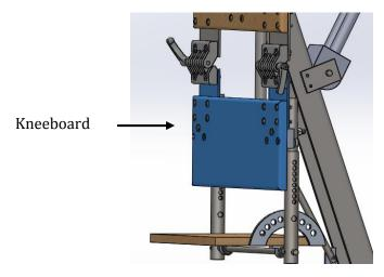
Figure 23: The kneeboard supports the lower half of the user's legs.
