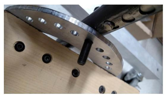
Figure 45: Arch-Shaped Pin Locking Mechanism.
