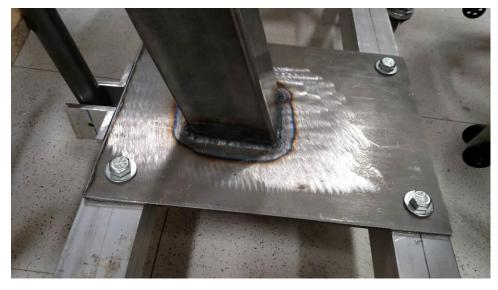
Figure 40: Base Plate Assembly.
