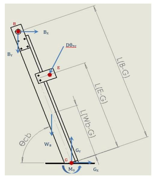
Defined Variables: W<sub>B</sub> = Weight of center beam of center beam
