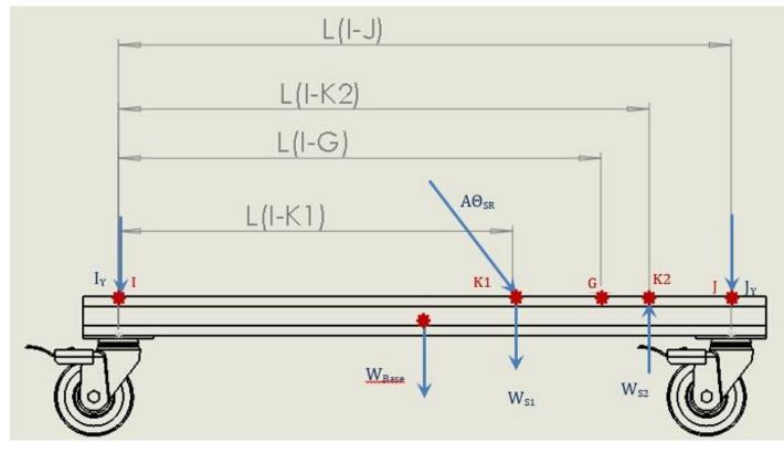
Defined Variables: W<sub>Base</sub> = Weight of base middle beam 1 W<sub>S1</sub> = Load due to
