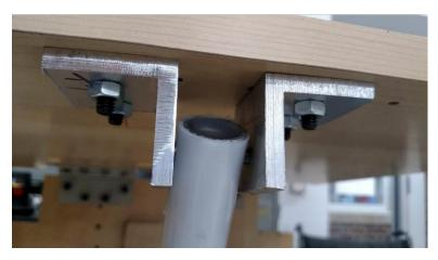
Figure 47: L Brackets and Tray Connection.
