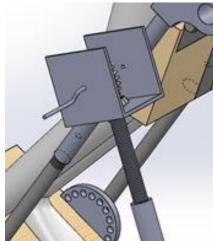
Figure 12: Gearbox can be manually operated with a handle to drive the lead screw.
