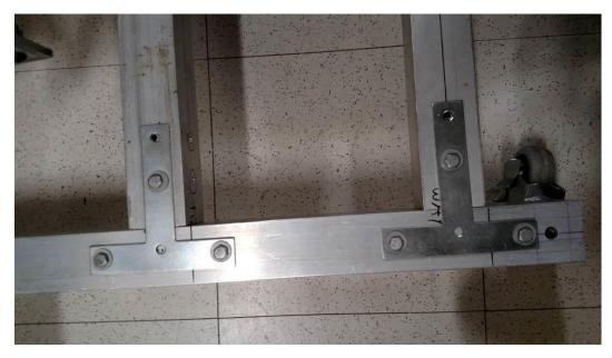
Figure 39: T-Bracket Assembly.
