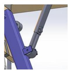
Figure 13: The slider's length can be adjusted to change the inclination of the tray.
