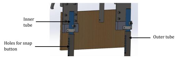
Figure 31: Telescoping tubes connecting the footboard with the kneeboard.
