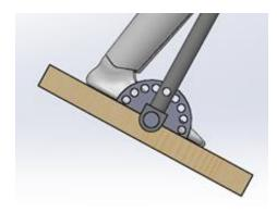
Figure 15: Footboard can pivot around an axis to enable ankle flexion.
