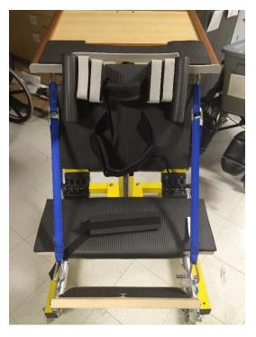
**Figure 46 Lateral Supports to Secure User**
