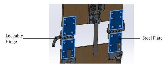
Figure 28: Lockable hinges and steel plates are used to connect the front and kneeboards.
