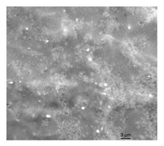
Figure 2. SEM photograph of strach-g-PVA/HA hydrogel (scale bar 3  $\mu m)$
