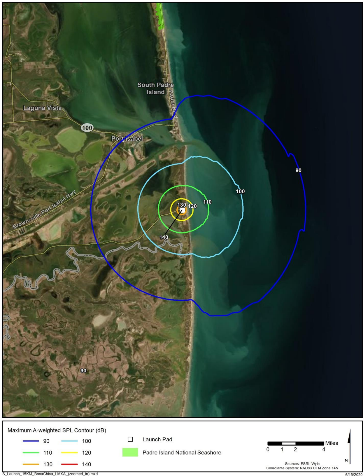
Figure 10. Starship Suborbital Launch from Boca Chica: Maximum A-Weighted Sound Levels (Zoom In)
