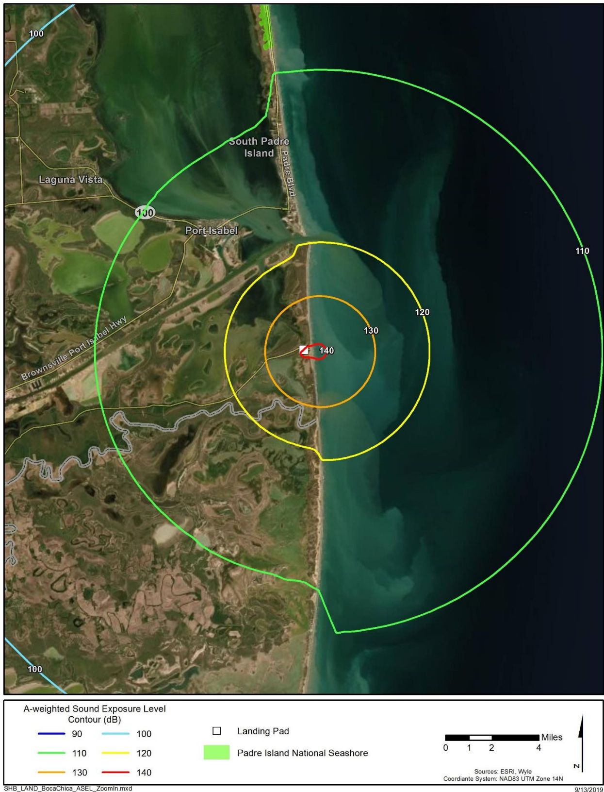
Figure 24. Super Heavy Booster Landing at Boca Chica: Sound Exposure Levels (Zoom in)
