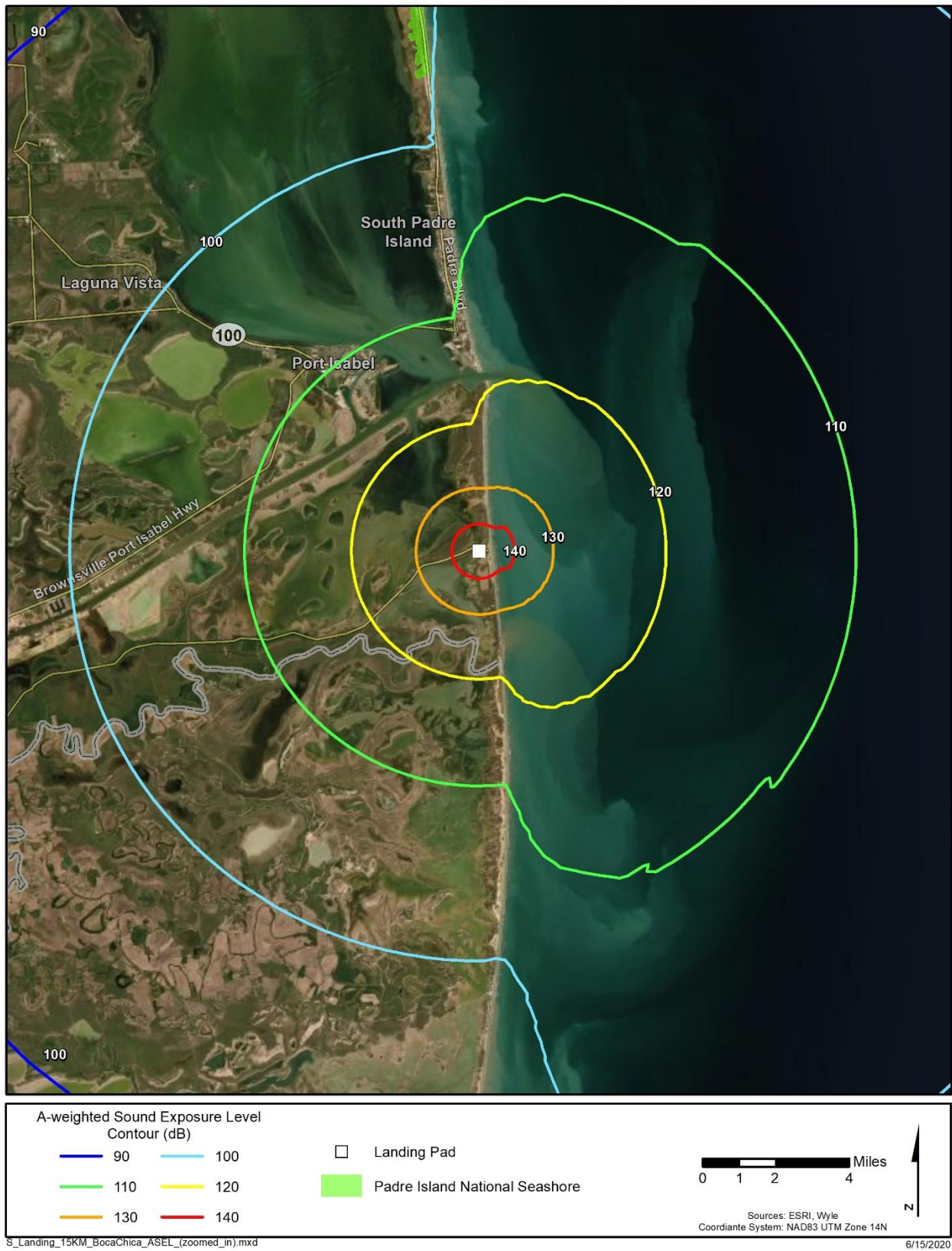
Figure 20. Starship Suborbital Flight Landing at Boca Chica: Sound Exposure Levels (Zoom In)
