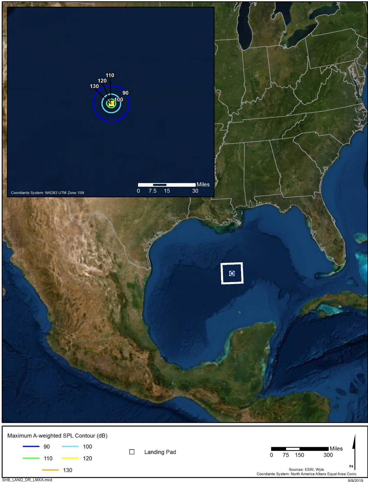
Figure 25. Super Heavy Booster Landing at the Downrange Site: Maximum A-Weighted Sound Levels
