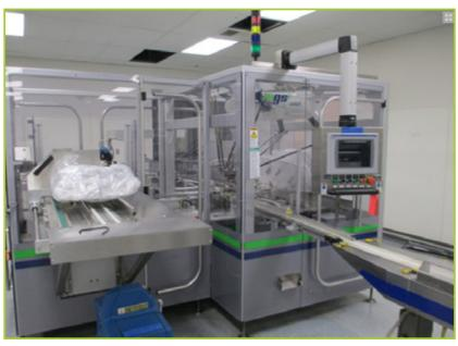
MGS MODEL TLC PICK AND PLACE ROBOTIC PACKAGING MACHINE
