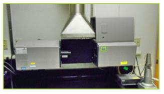
MALVERN MASTERSIZER-S (MSS) LASER PARTICLE SIZE ANALYZER
