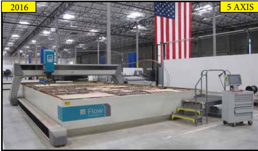
2016 FLOW MODEL M4C 4080 XD 049104-3, 5 AXIS CNC WATERJET CONTOUR MACHINE S/N 131202, FLOW CNC CONTROLS, FLOW DYNAMIC XD 5 AXIS END EFFECTOR CUTTING HEAD, FLOW MDL 058007-1 94 KSI PUMP UNIT, FLOW GARNET HOPPER, 190" X 348" TABLE, FILTRATION SYSTEM, 1361 HOURS.
