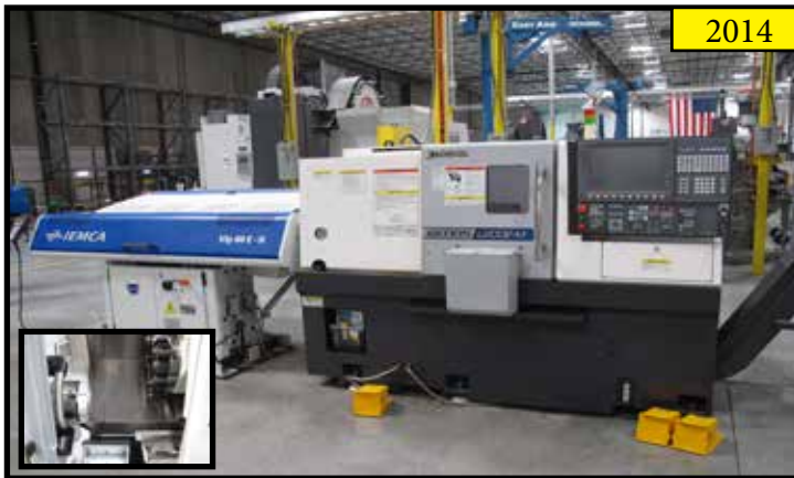
2014 OKUMA GENOS L200E-M CNC TURNING CENTER, LIVE TURRET, 8" CHUCK, 2.6" THRU SPINDLE, 17.72" SWING OVER BED, 13.78" SWING OVER CROSS SLIDE, 6000 RPM ON LIVE TOOLING, 12 STATION TURRET, OKUMA OSP-P300 L-R CONTROL, TOOL PRESETTER, HYD TAILSTOCK, PARTS CATCHER, CHIP CONVEYOR, S/N ME837,
