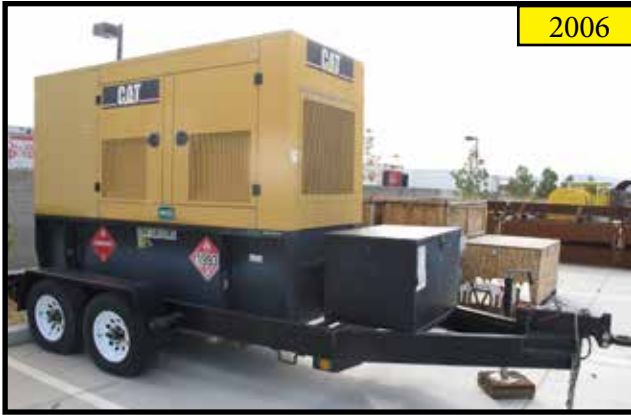
2006 CATERPILLAR D150-8 PORTABLE DIESEL GENERATOR, 150 KW, S/N CAT00C66VSDA00421, WITH EMCP301 CONTROLS, TRAILER, (BILL OF SALE ONLY)
