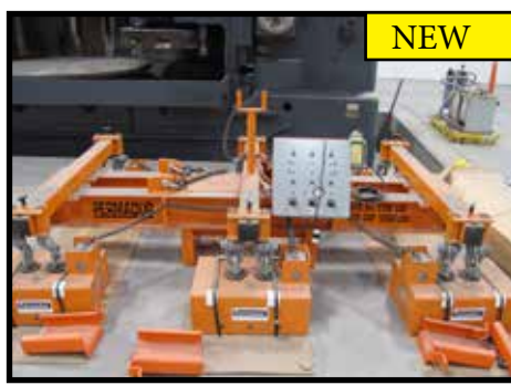
PERMADUR 12,000 LB CAP MAGNETIC LIFT SYSTEM. (NEW)
