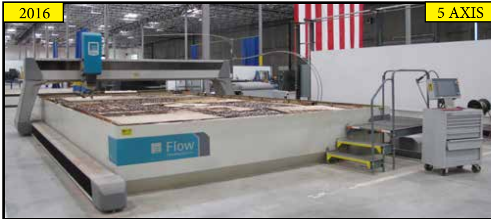
2016 FLOW MODEL M4C 4080 XD 049104-3, 5 AXIS CNC WATERJET CONTOUR MACHINE S/N 131202, FLOW CNC CONTROLS, FLOW DYNAMIC XD 5 AXIS END EFFECTOR CUTTING HEAD, FLOW MDL 058007-1 94 KSI PUMP UNIT, FLOW GARNET HOPPER, 190" X 348" TABLE, FILTRATION SYSTEM, 1361 HOURS.
