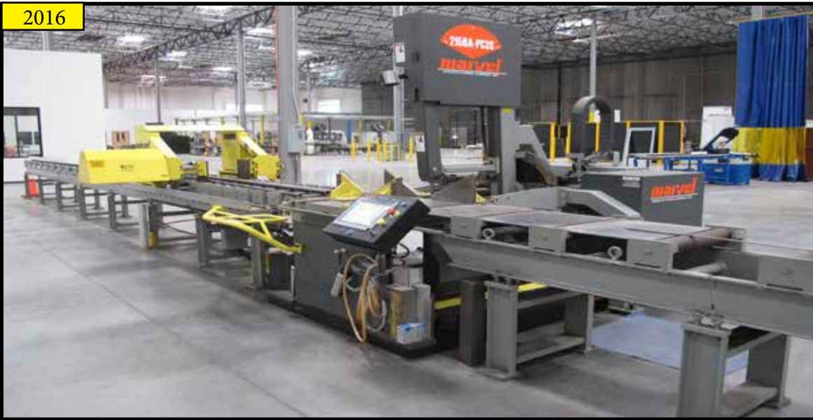
2016 MARVEL 2150A-PC3S MODEL F2150PC3S VERTICAL TILT FRAME CNC BAND SAW, WITH SIEMENS PC3 SAW CONTROL, HYD CLAMPING AND AUTO FEEDS, PLUS AND MINUS 60 DEGREE CUTING ANGLES, BUNDLE CLAMPING ACCESSORY, CONVEYOR, S/N F2150-20346-PC3S.
