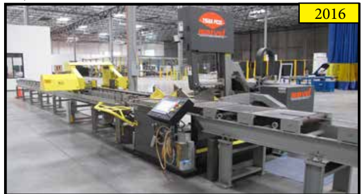
2016 MARVEL 2150A-PC3S MODEL F2150PC3S VERTICAL TILT FRAME CNC BAND SAW, WITH SIEMENS PC3 SAW CONTROL, HYD CLAMPING AND AUTO FEEDS, PLUS AND MINUS 60 DEGREE CUTTING ANGLES, BUNDLE CLAMPING ACCESSORY, CONVEYOR, S/N F2150-20346-PC3S.
