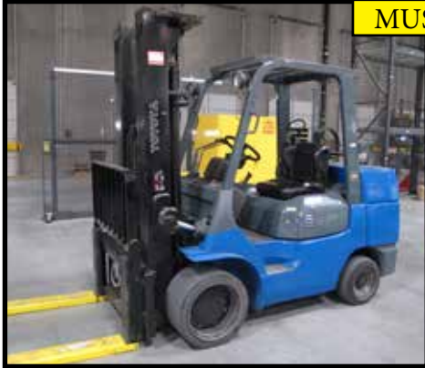
TOYOTA 7FRGU45, 10,000 LB CAP LPG FORKLIFT, 3 STAGE MAST, 187" LIFT HEIGHT, CUSHION TIRES, 6560 HOURS (APPROXIMATE), S/N 70247.
