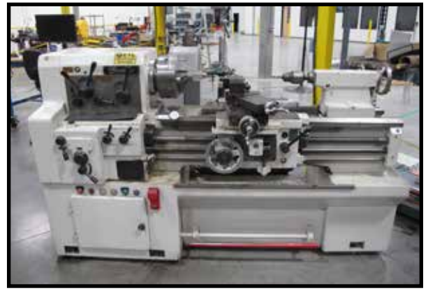
CADILLAC 1733, 17" X 33" GEARED HEAD GAP ENGINE LATHE, 32 - 1800 RPM, INCH THREADING, 10" 3 JAW CHUCK, S/N 868648.
