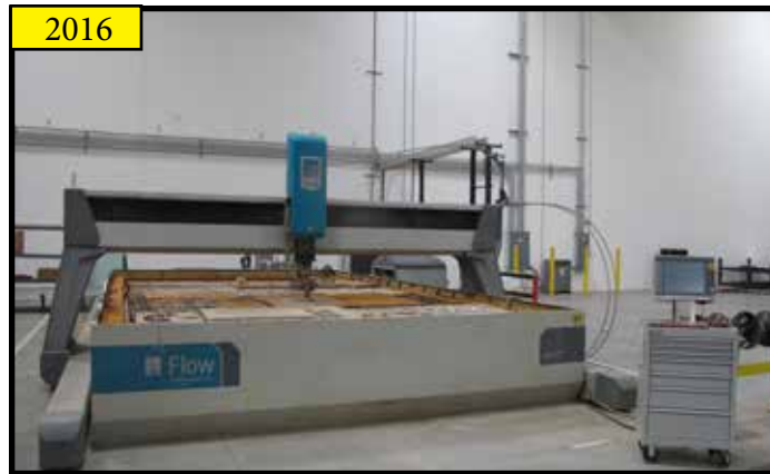
2016 FLOW "MACH 4 4080C" MODLE M4C 4080 DWJ 049104-3 CNC WATERJET CONTOUR MACHINE, S/N 131200 WITH FLOW CONTROLS, FLOW HYPERJET MDL 058007-1 94 KPSI PUMP UNIT, FLOW GARNET HOPPER, EBBCO TEAEVO TECH CLOSED LOOP CHILLER UNIT, EBBCO WJF-2004-CD FILTRATION SYSTEM, 190" X 348" TABLE, 1105 HOURS.
