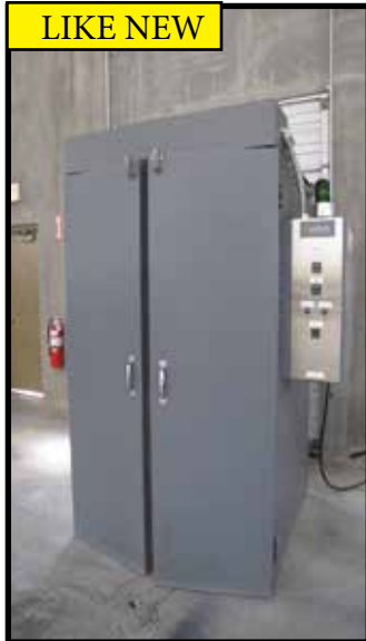
2016 JPW INDUSTRIES MODEL ST496TULF480V30KW WALK IN ELECTRIC OVEN, 500 DEG F MAX, DIGITAL CONTROL, DOUBLE DOORS, 48"W x 72"H x 42" DEEP.
