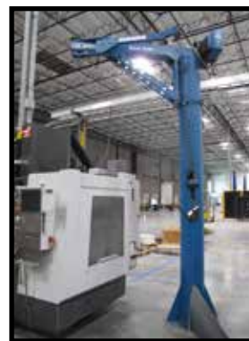
(3) GORBEL "EASY ARM" 330 LB AND 660 LB CAP INTELLIGENT LIFTING SYSTEM, FLOOR MOUNTED JIB CRANE, W/ G-FORCE 330 LB AND 660 LB CAP ELECTRIC HOIST
