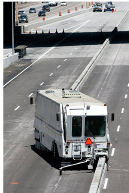
Figure 2 – Movable Barriers of I-15 in San Diego
