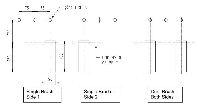
Note: Belt direction is not critical. The cleaner is suitable for reversing belts.
