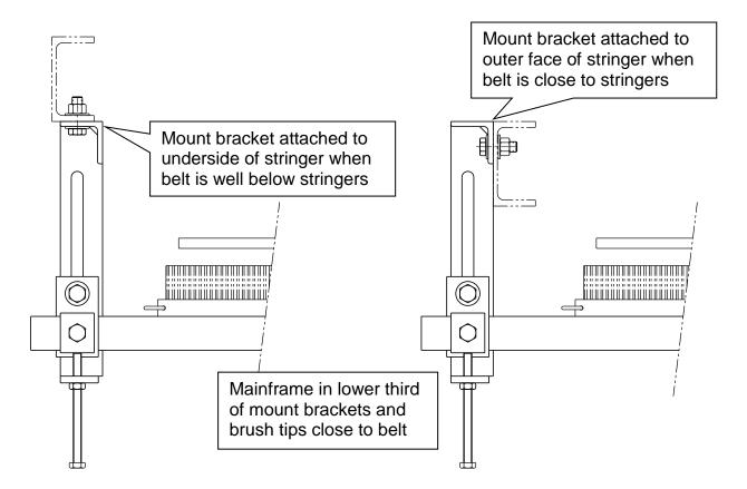
Mount bracket attachment is determined by the belt height in relation to the stringers.
