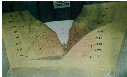
Photo 4. The failure mode of the model from Downstream
