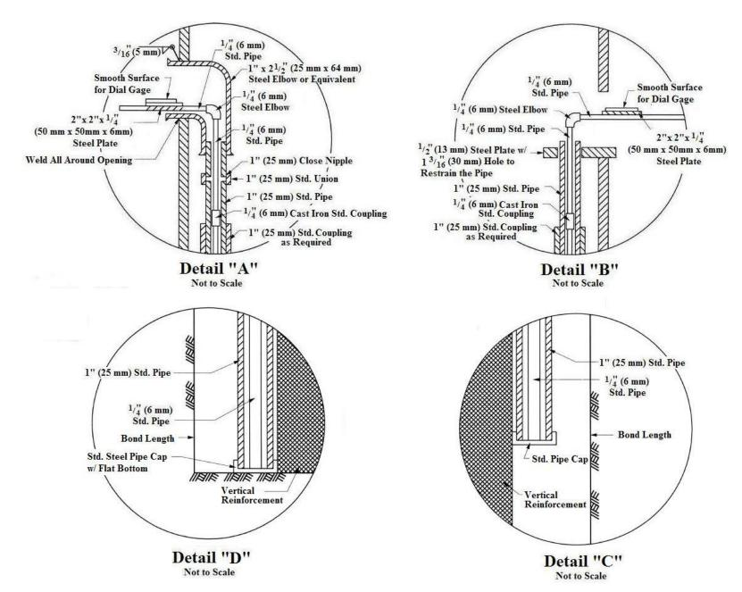
Figure 12 Dial Support and Telltale Attachment Details for Micropiles
