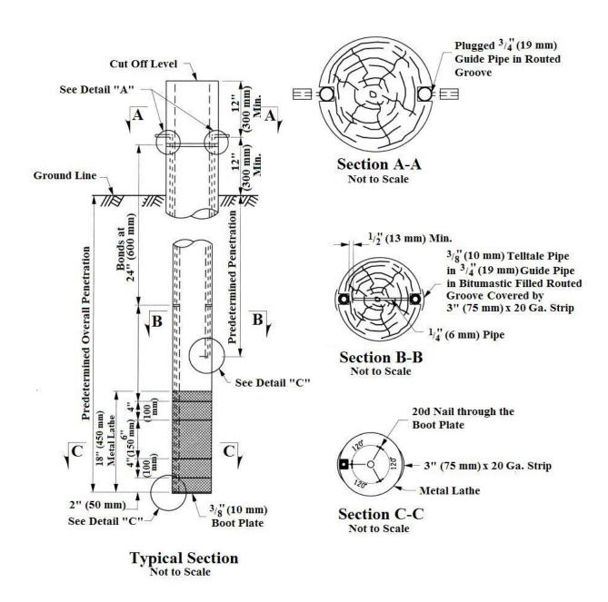
Figure 13 Telltale Installation Details for Timber Piles
