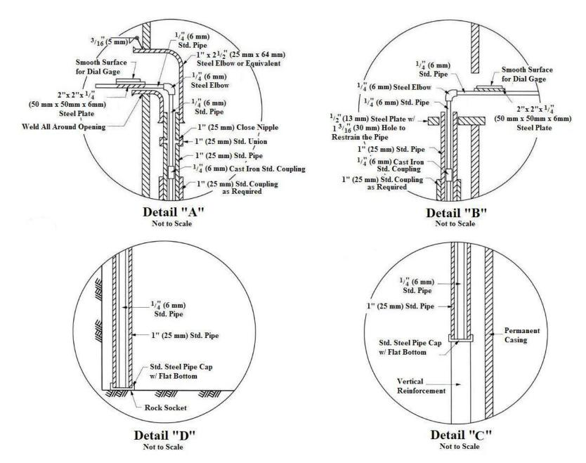
Figure 10 Dial Support and Telltale Attachment Details for Drilled Shafts
