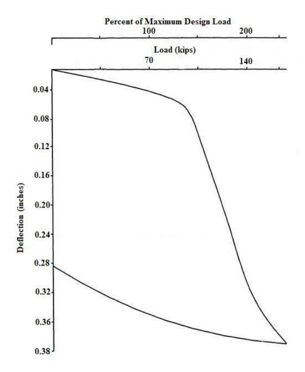
Figure 20 (a) Typical Load vs. Deflection Plot for Constant Rate of Penetration Test (US Customary Units)
