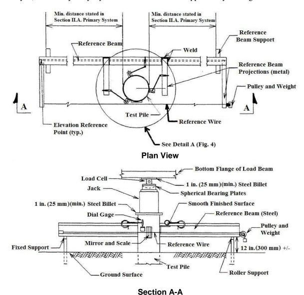
Figure 3 Typical Setup for Measuring System
