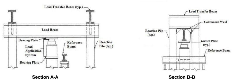
Figure 1 Typical Setup for a Reaction Frame
