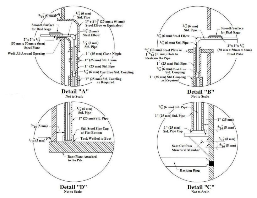
Figure 8 Dial Support and Telltale Attachment Details for Pipe Piles
