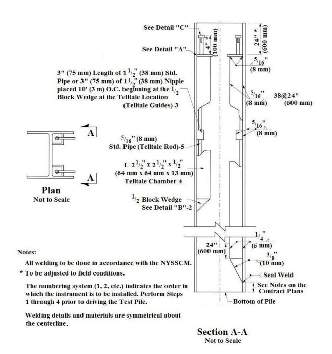
Figure 5 Telltale Installation Details for H-Piles
