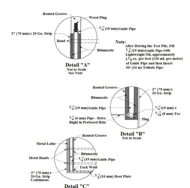
Figure 14 Dial Support and Telltale Attachment Details for Timber Piles
