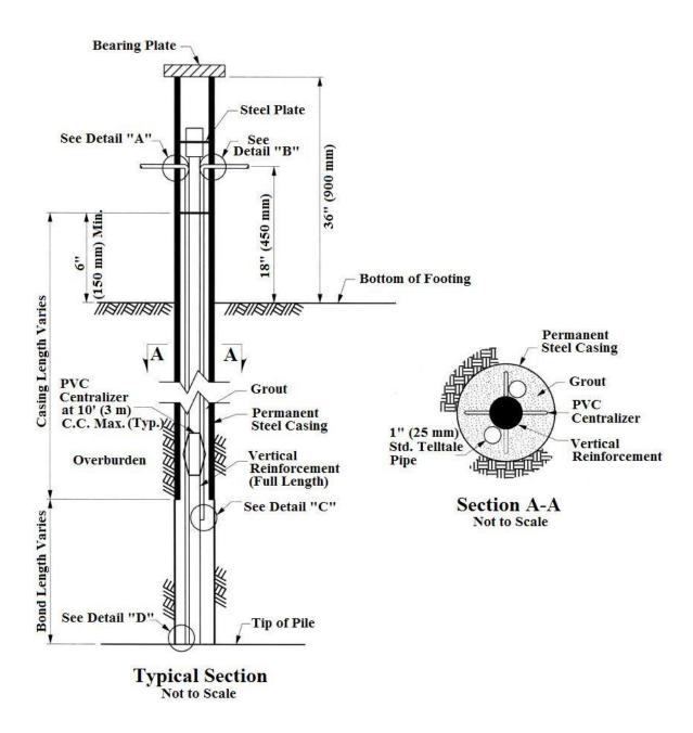
Figure 11 Telltale Installation Details for Micropiles
