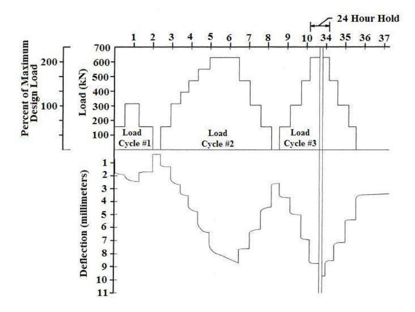
Figure 19 (b) Typical Load-Deflection vs. Time Plot for Incremental Static Load Test (International System of Units)
