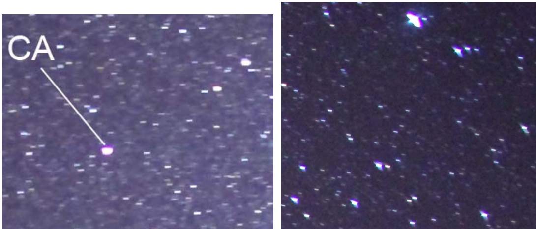
100% Views: Chromatic Aberration (CA) and “Seagulls” (Canon 5D + Canon 24mm f/1.4L II lens)
