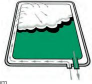
STATIM uses clean water with every cycle, preventing the formation of rust and the build-up of bio contaminants. If incorrect water is used, the STATIM will not start the cycle and will display a warning.
