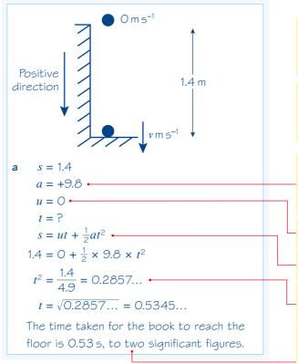
Model the book as a particle moving in a straight line with a constant acceleration of magnitude  $9.8 \text{ m s}^{-2}$ .
