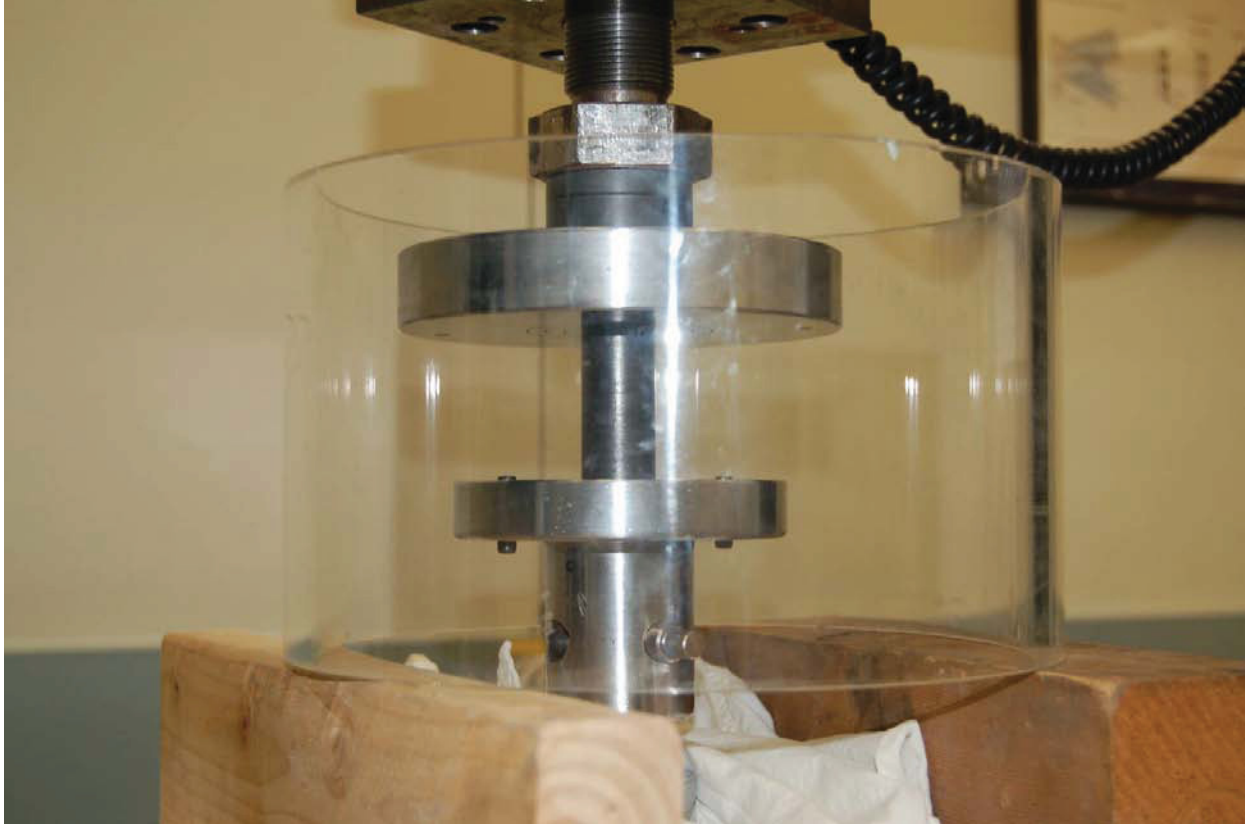
Figure 3. Compressive strength test configuration.
