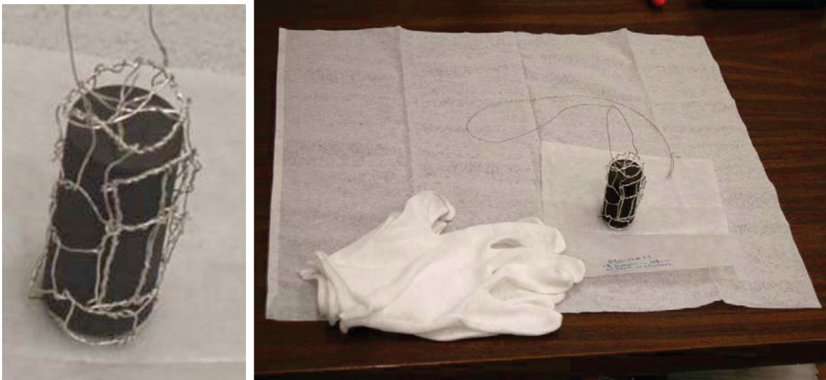
Figure 2. Suspension wire and basket with graphite sample.
