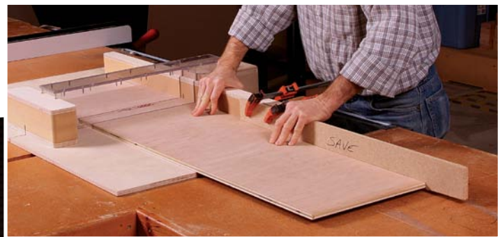
Set the stop. The long MDF auxiliary fence lets you set up a stop at the far end for cutting a series of workpieces to the same length.
