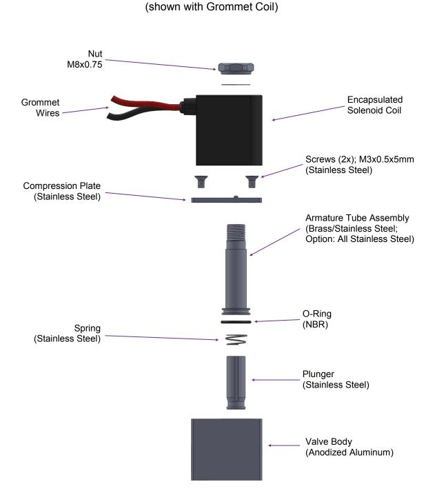
**2V025 Series Solenoid Valve Components**
