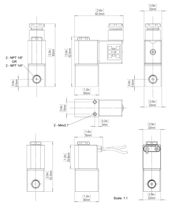
**Note:** Dimensions shown with DIN Connection above & Grommet Connection below. Dimensions are for reference only. Field verify dimensions prior to installation for critical dimensions.
