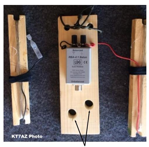
Cable runs through holes for strain relief
