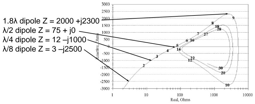
Feed-point impedance versus frequency for a theoretical 100-foot long dipole in free space, fed in the center and made of extremely thin 0.001-inch diameter wire. (Source: ARRL Antenna Book)
