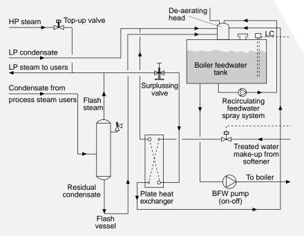
Figure 5: Flash steam recovery system and feedwater tank.
