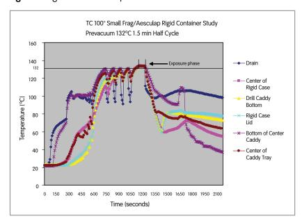
Figure 2: Rigid Container Temperature Profile
