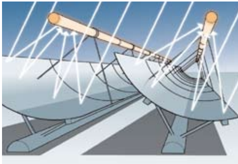
Parabolic trough collectors
