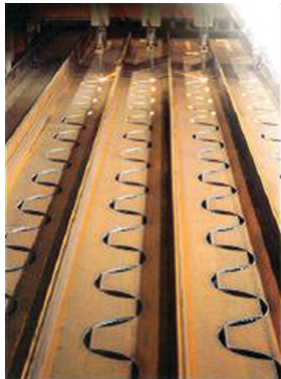
Fig. 1-4. Second cutting of a cellular pattern.
