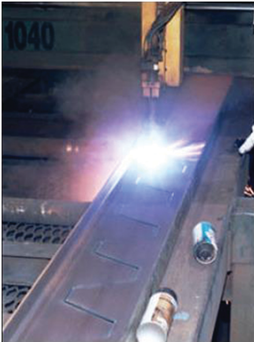
Fig. 1-2. Cutting of a castellated pattern.
