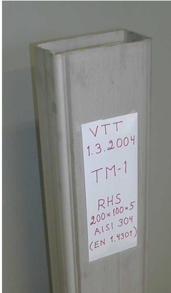
Figure 8. Test material TM-1 (cold-formed 200 x 100 x 5 rectangular hollow section made of stainless steel).
