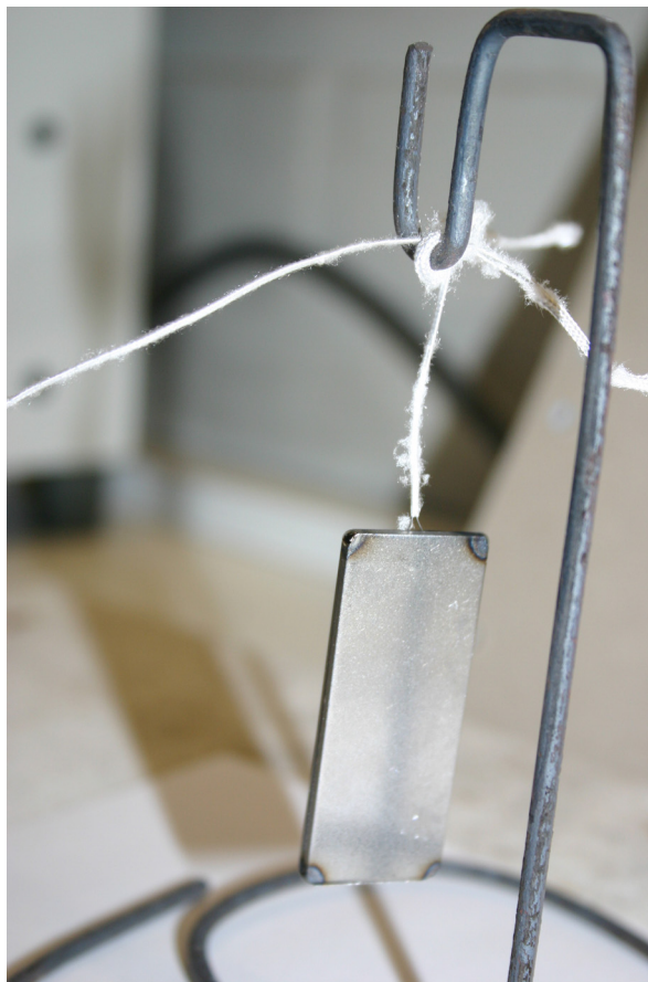
Figure 12. A photograph of test specimen TM-3-6 hanging from the specimen holder on a thermocouple. Color changes in the corners of the test specimen are due to welding.
