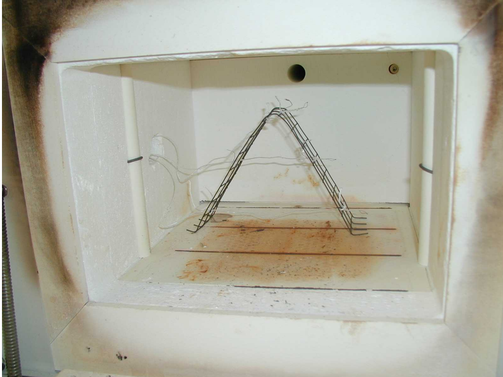
Figure 13. The thermocouples and thermocouple holder for the measurement of the air temperature inside the furnace chamber.
