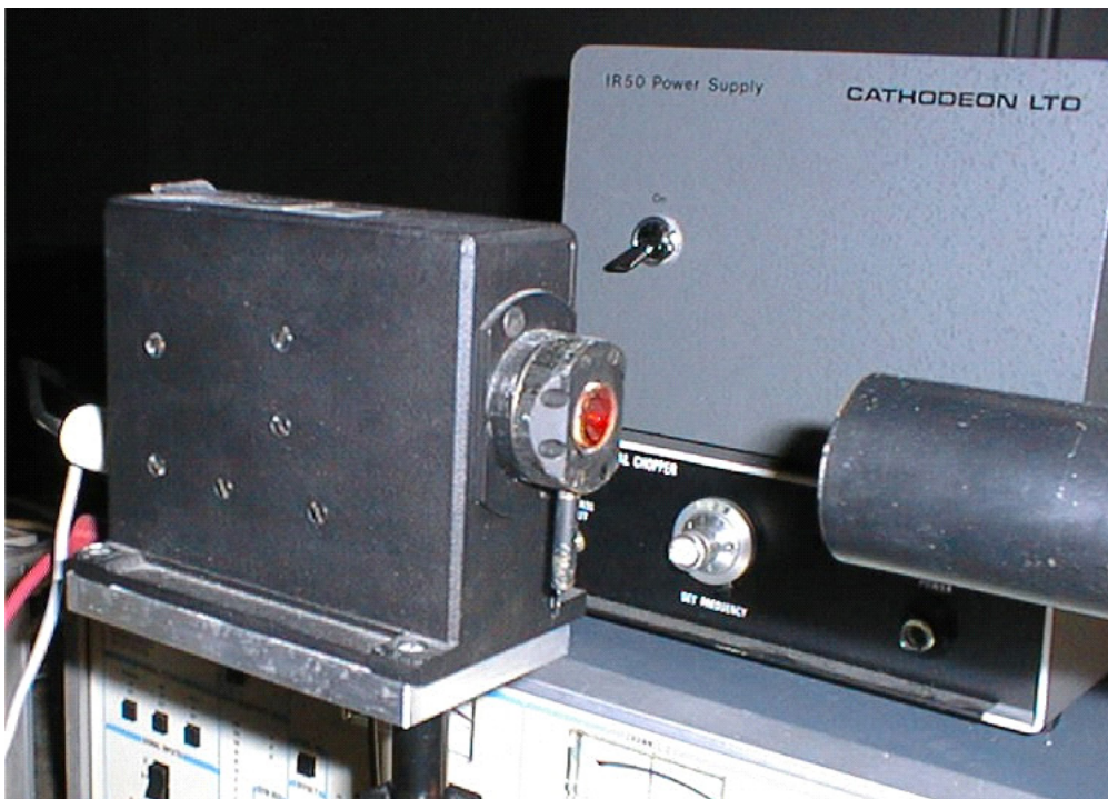
Figure 39. The Golay detector with its reddish KRS5 window. It is inserted into the tube seen to the right.
