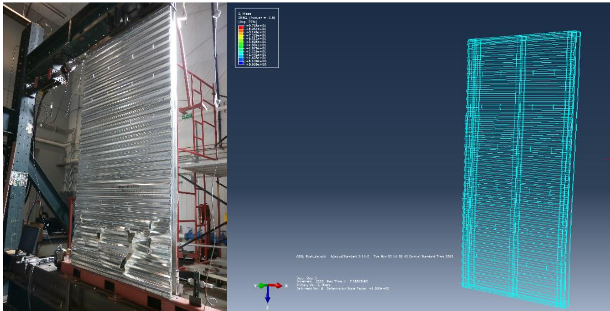
Figure 70 - Model 3: sheathing deformation
