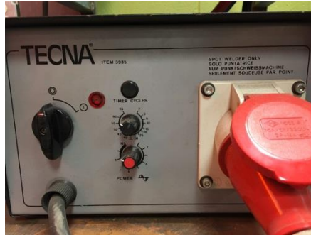
Figure 12 - Spot-welding power supply
