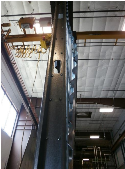
Figure 48 - Unzipping of spot-weld connections
