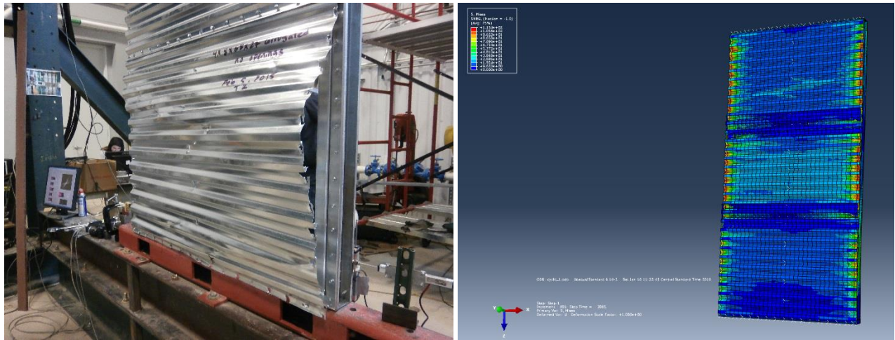
Figure 66 - Model 2: sheathing deformation
