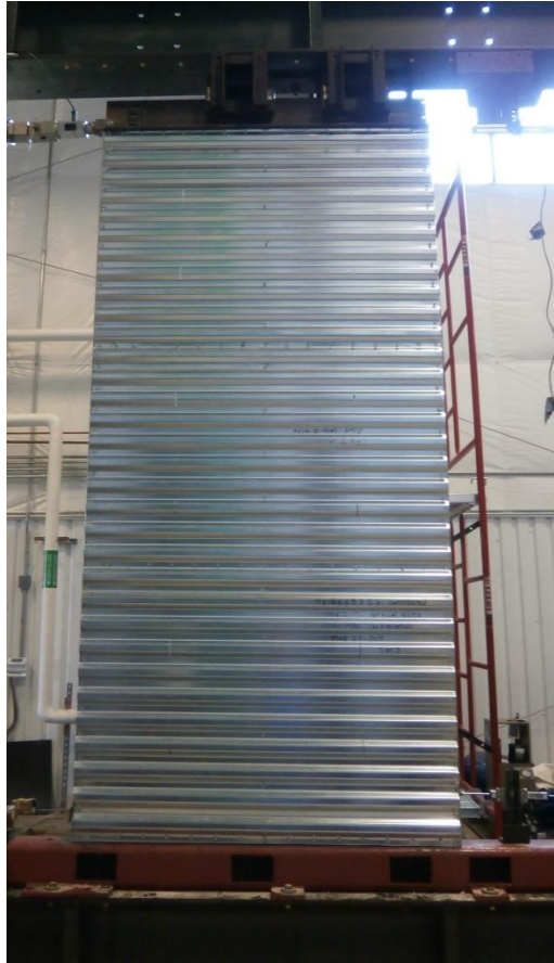
Figure 9 - Sheet out wall configuration
