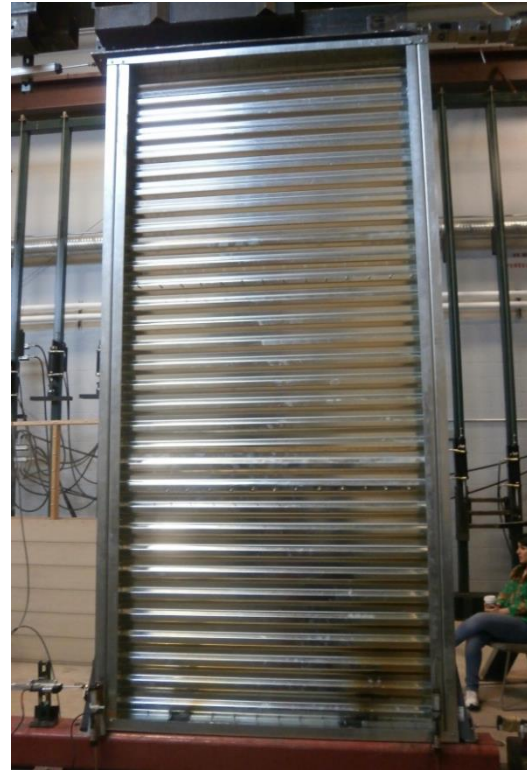
Figure 14 - Sheet in wall configuration (back view)
