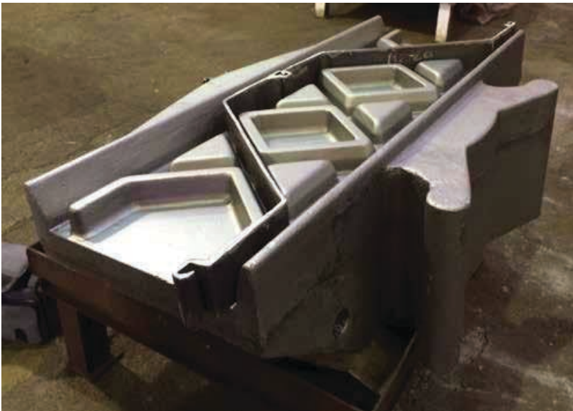
Typical driving cap for Z-sheet piles
